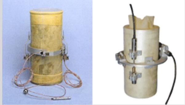
**Fig. 7 Hall Effect and LVDT local strain transducers**
