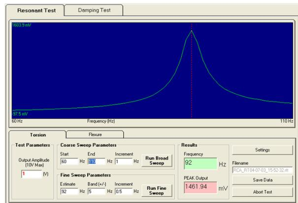
Fig. 1 GDS RCA software resonance test data
