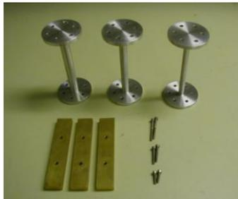
**Fig. 5 Calibration bars and weights**
