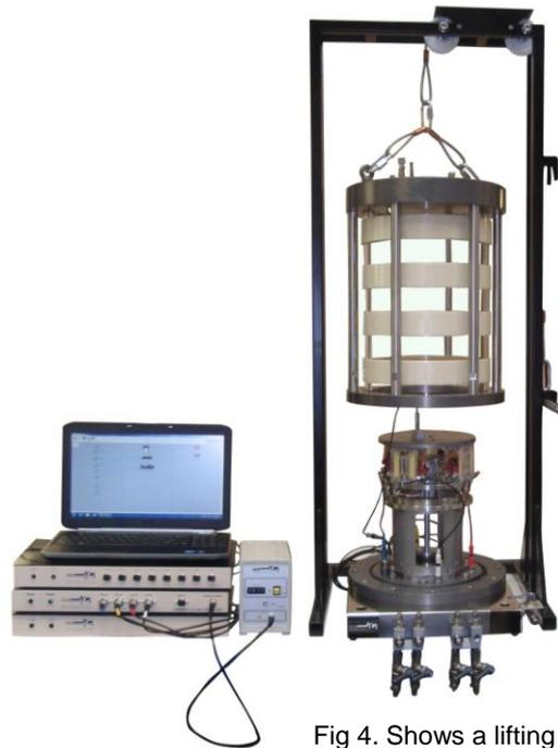
Fig 4. Shows a lifting frame for the resonant column
