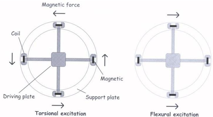
Fig. 3 Drive schematic for torsional and flexural excitation
